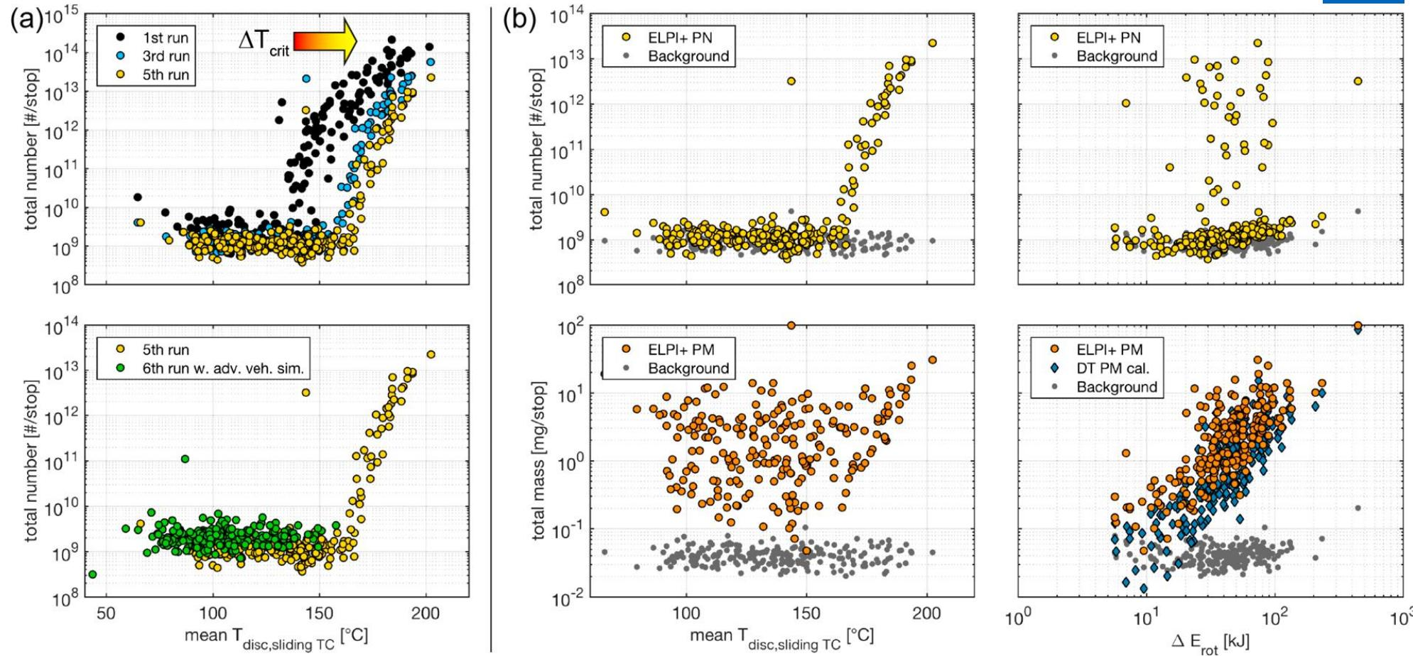
**Particle mass - non-linear increase with energy dissipated**
